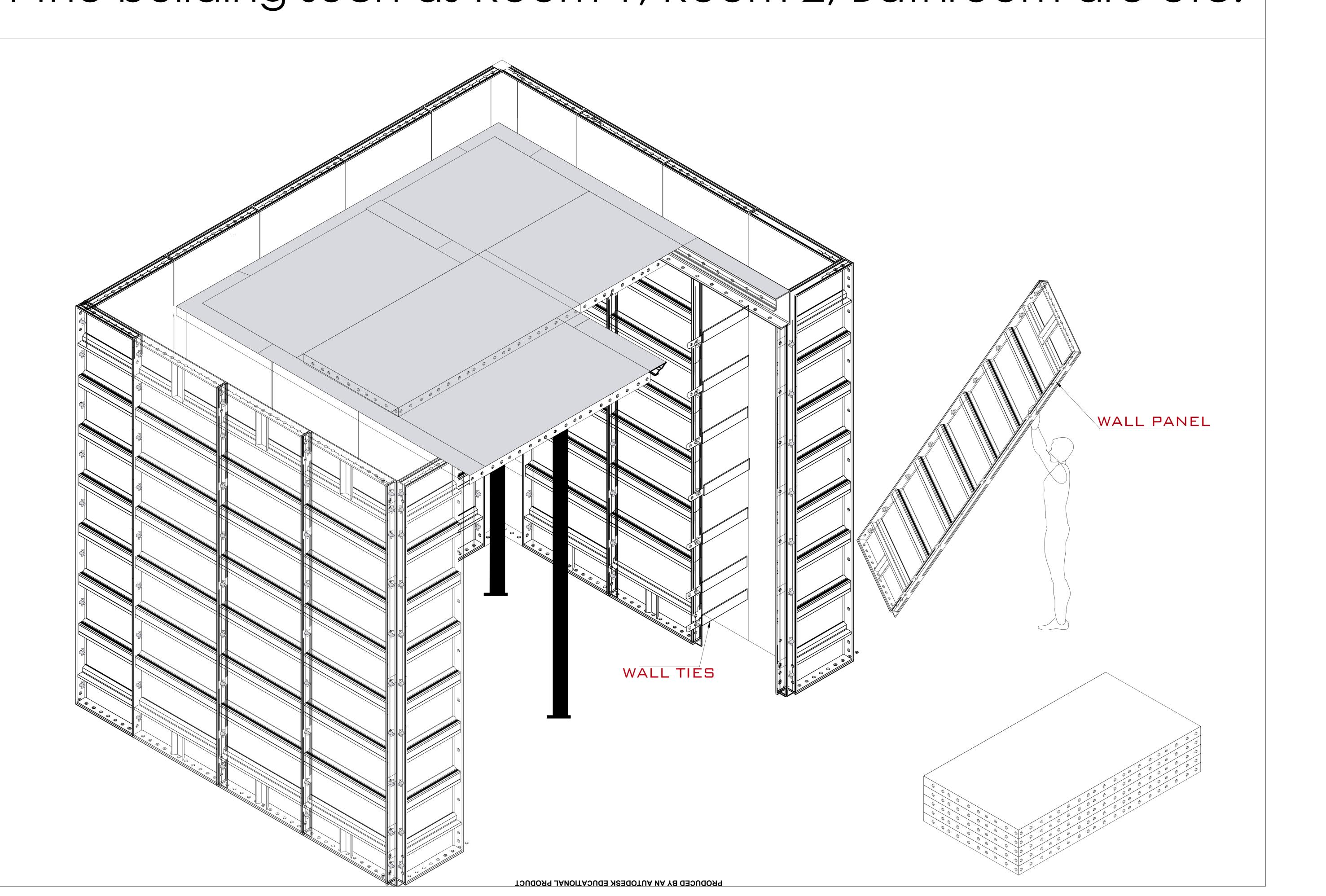
After removing the External Wall Forms (the starter Block (kicker) should remain undisturbed), the dismantled wall forms are moved to upper floor. Access Scaffolding is use for transferring of external wall panels from the ground floor level. For level 1 and above, an external working platform is fixed to the external wall. The external wall forms from level 1 onward shall be supported by the kickers. (These steps are to be repeated from one floor to another floor.)
