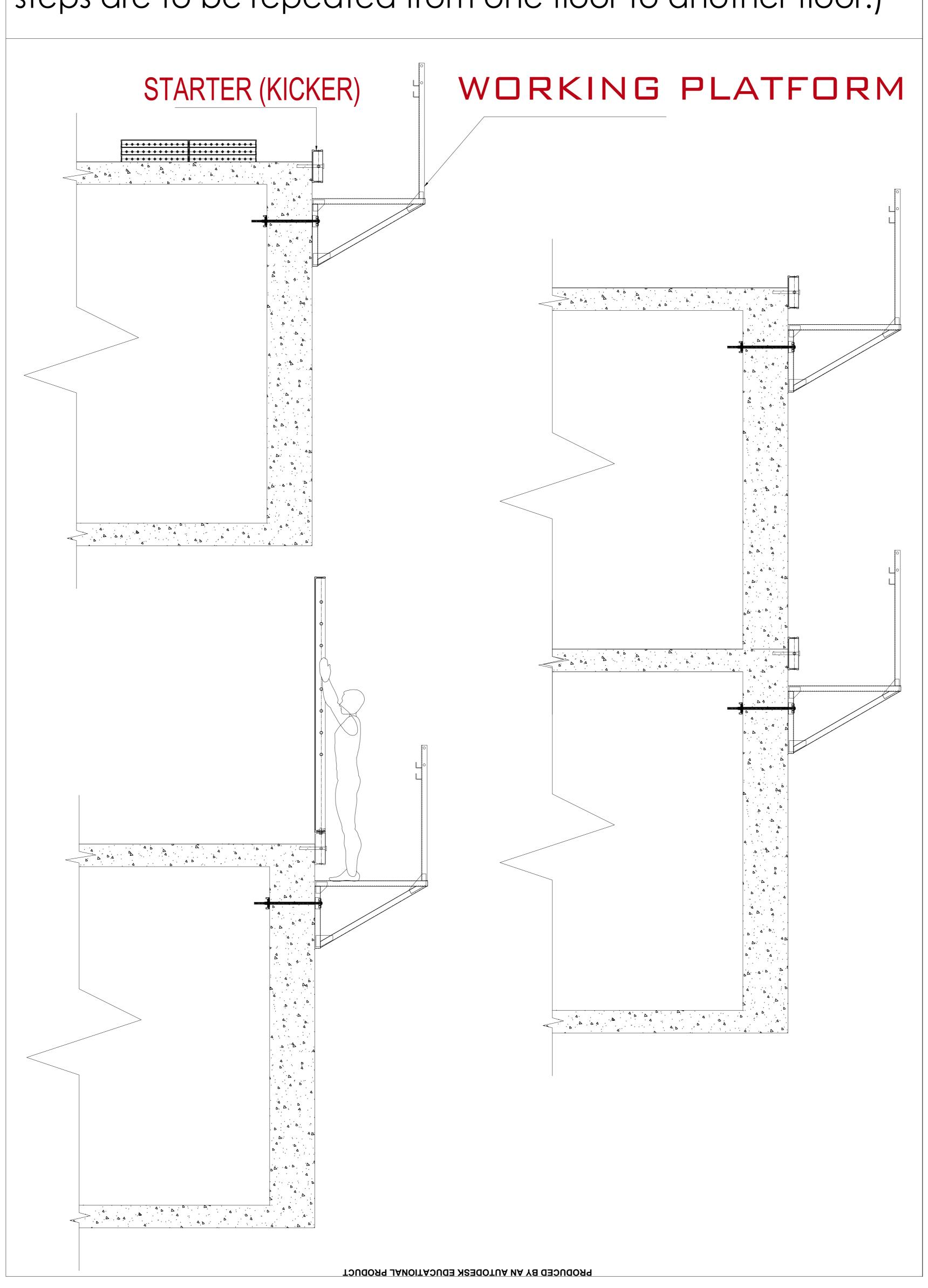
After removing the Wall Panels, proceed to the Slab Panels after 36 hours by removing the long pins and wedges on the joint bars the end and middle beam section.
